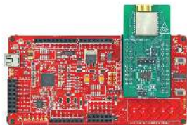
Fig 4: Programming and debugging with CY8CKIT-042-BLE BLE Pioneer Kit Baseboard
