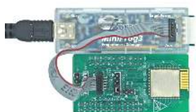
Fig 3: Programming/Debugging with MiniProg3
