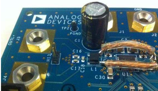
Figure 3. Board Modifications for Mono Mode
