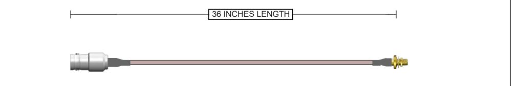
Connector A 112631 BNC Jack Straight Brass Nickel + Heatshrink 50 Ohm RG-178 Continuity/Hi-Pot Connector B 132286 SMA Jack Straight Bulkhead - Rear Mount Brass Gold + Heatshrink
