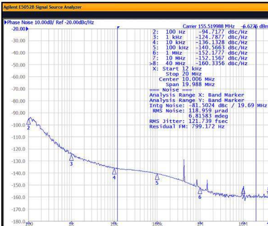
Figure 8.3. Input = 25 MHz; Output = 155.52 MHz, 2.5 V LVDS
