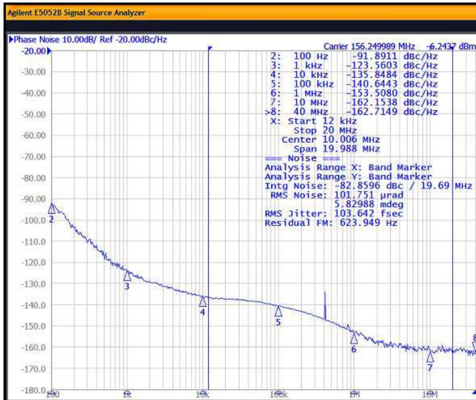
Figure 8.2. Input = 25 MHz; Output = 156.25 MHz, 2.5 V LVDS
