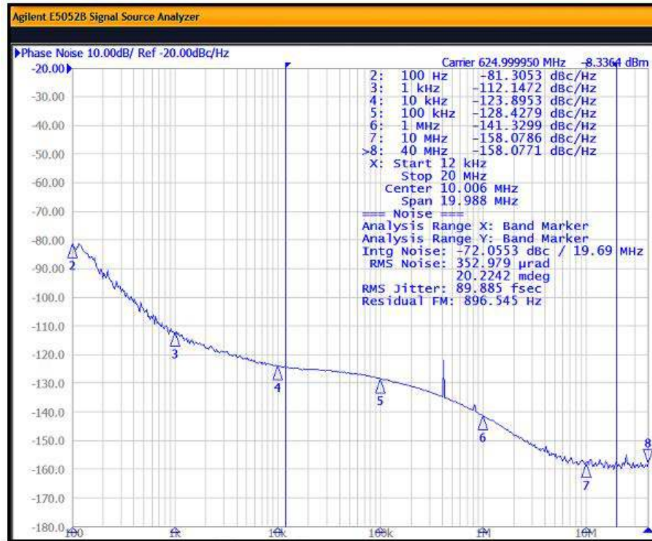
Figure 8.1. Input = 25 MHz; Output = 625 MHz, 2.5 V LVDS
