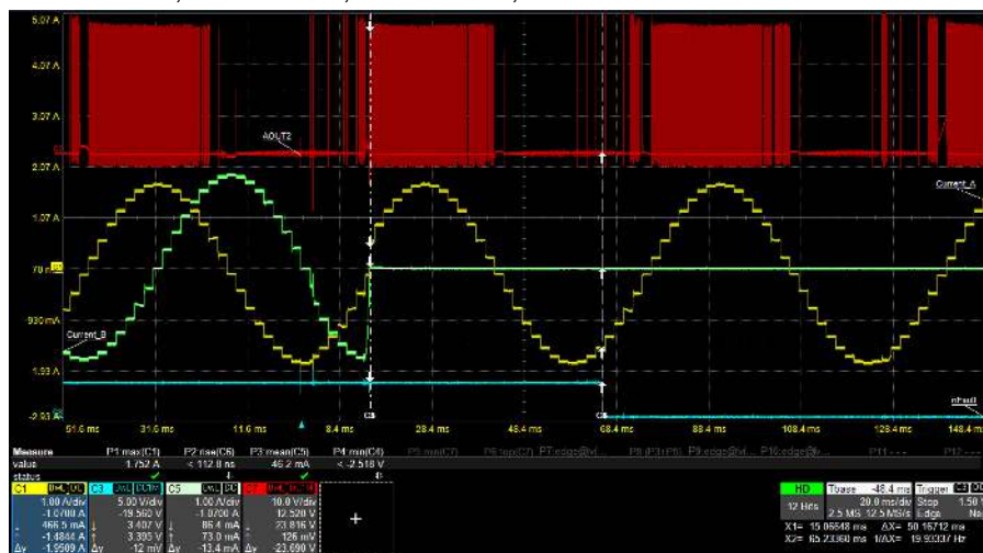
Figure 7-46. Coil B open-load detection
