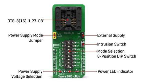
However, the Secure SOIC click is designed in a way that every IC from the CryptoAuthentication<sup>™</sup> family from Microchip is fully supported with all of its features. Due to many different ICs and possibilities supported, the only way for achieving such a goal was to use the 8-positions DIP switch. That way, user is able to select the communication lines routed the way it is required for any application.
