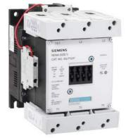
Vacuum NEMA contactor, Size 5, Three phase full voltage, Contactor amp rating 270A, 3 wire (NO aux included), 575-600V 50-60Hz/DC coil, Non-combination type, Enclosure NEMA type (open), No enclosure
