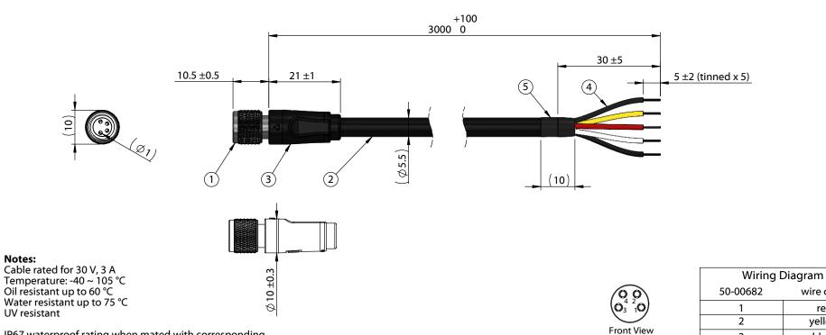
IP67 waterproof rating when mated with corresponding (IP67) connector
