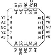
SN54367A, 368A, SN54LS367A, 368A . . . J PACKAGE **SN74367A, 368A...N PACKAGE** SN74LS367A, SN74LS368A . . . D OR N PACKAGE (TOP VIEW)
