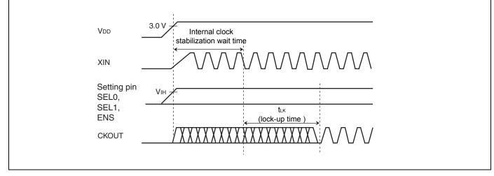
If the setting pin is fixed at the "H" or "L" level, the maximum time after the power is turned on until the set clock signal is output from CKOUT pin is (the stabilization wait time of input clock to XIN pin) + (the lock-up time " $t_{LK}$ "). For the input clock stabilization time, check the characteristics of the resonator or oscillator used.
