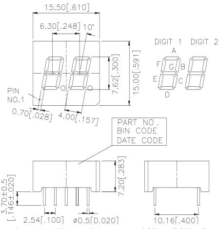
NOTES: All dimensions are in millimeters. Tolerances are ± 0.25 mm (0.01") unless otherwise noted.
