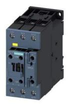
power contactor, AC-3e/AC-3, 51 A, 22 kW / 400 V, 3-pole, 21-33 V AC/DC, 50/60 Hz, with integrated varistor, auxiliary contacts: 1 NC, screw terminal, size: S2, F-PLC-IN
