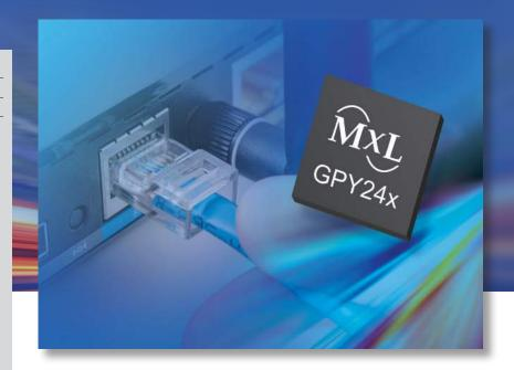
Faster Ethernet connectivity enables users to make the most of increased speeds available through the enhanced broadband access networks. 2.5Gigabit Ethernet (GbE) increases the bandwidth without the need to change cables, is more cost-effective, and consumes less power than 5GbE or 10GbE.
