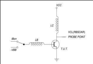
Fig.13. Test Circuit for reverse bias safe operating area.  $V_{cl} \leq 1000V$ ;  $V_{cc} = 150V$ ;  $V_{BB} = -5V$ ;  $L_B = 1\mu H$ ;  $L_c = 200\mu H$
