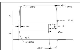
Fig.4. Switching times waveforms with resistive load.
