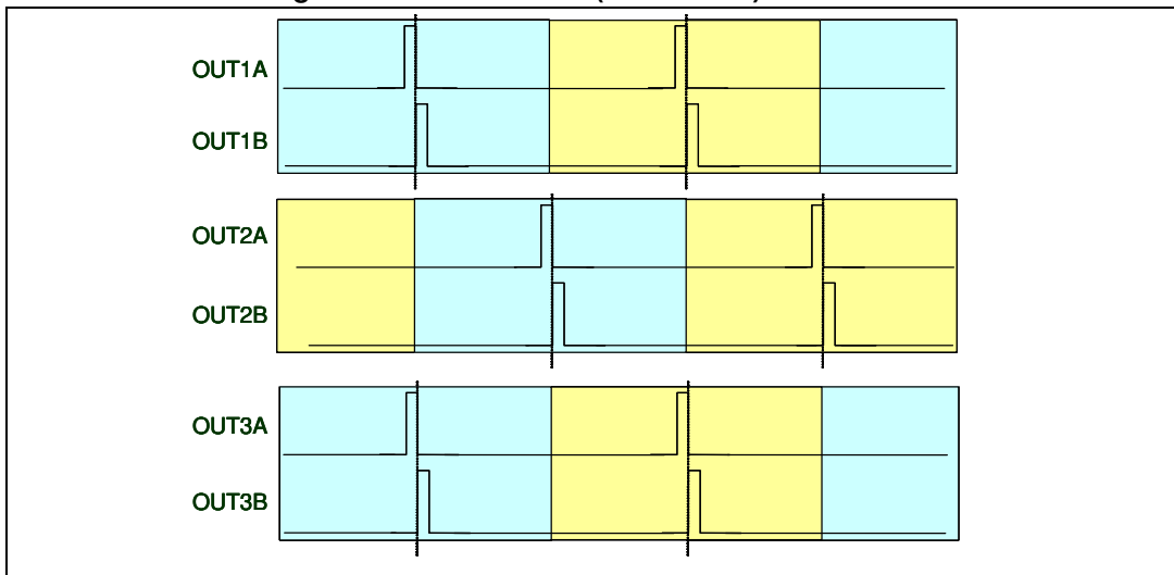
Figure 18. 2.1 channels (OCFG = 10) PWM slots
