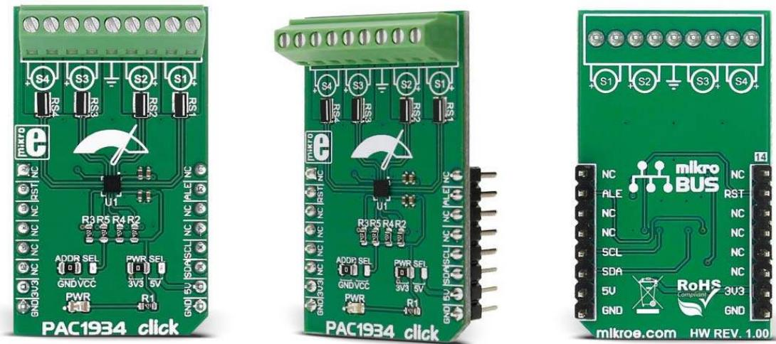
**PAC1934 click** carries the PAC1934 four channel DC power/energy monitor from Microchip. The click is designed to run on either 3.3V or 5V power supply. It communicates with the target microcontroller over an I2C interface.
