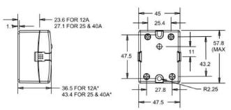
\* Overall height dimensions includes with clear cover Dimensions in mm
