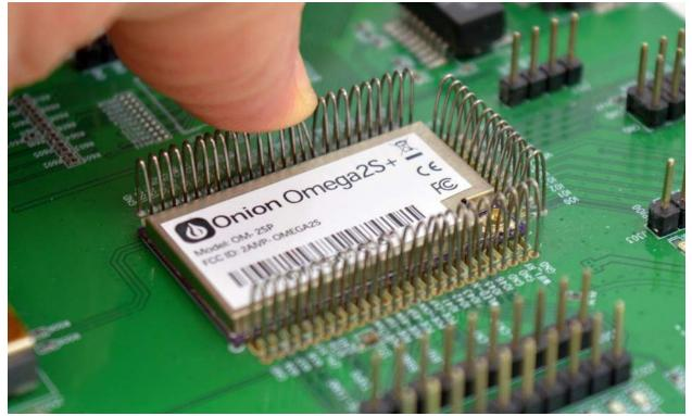
• Refer to our visual guide for more clarity on the combing procedure: <u>https://youtu.be/aoYadArVJPw</u>  Always check that each rail-pin is connected to its corresponding Omega castellated socket before powering the device. The image below represents the incorrect positioning of the rail-pin:
