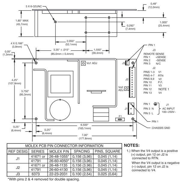
Figure 1. Mechanical Drawing
