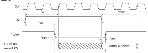
21. The IGNORE CLOCK EDGE or STALL cycle (Clock 3) illustrated CEN being used to create a pause. A write is not performed during this cycle. 22. Device must be deselected when entering ZZ mode. See cycle description table for all possible signal conditions to deselect the device.
