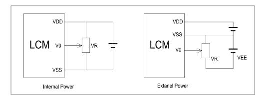
$V_{DD-}V_0$ : LCD Driving voltage VR: 10k~20k
