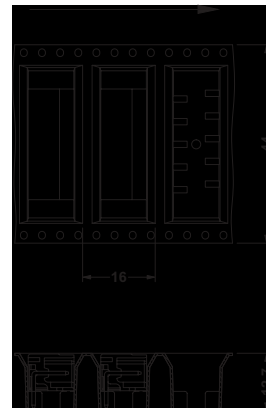
MC 0,5/...-G-2,5 THT R44, Tape width 44 mm, odd nos. of positions, feeder direction
