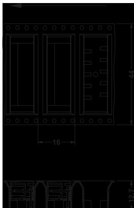
MC 0,5/...-G-2,5 THT R44, Tape width 44 mm, even nos. of positions, feeder direction
