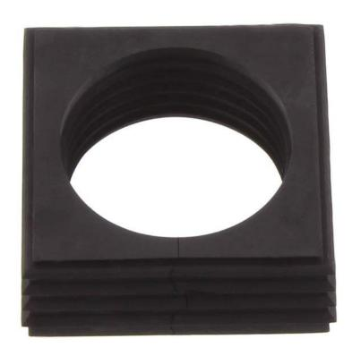
Seal, Mounting type: Plug in, Length x width: 42.8 mm, Max. cable diameter: 33 mm, IP 66, Colour: Black
