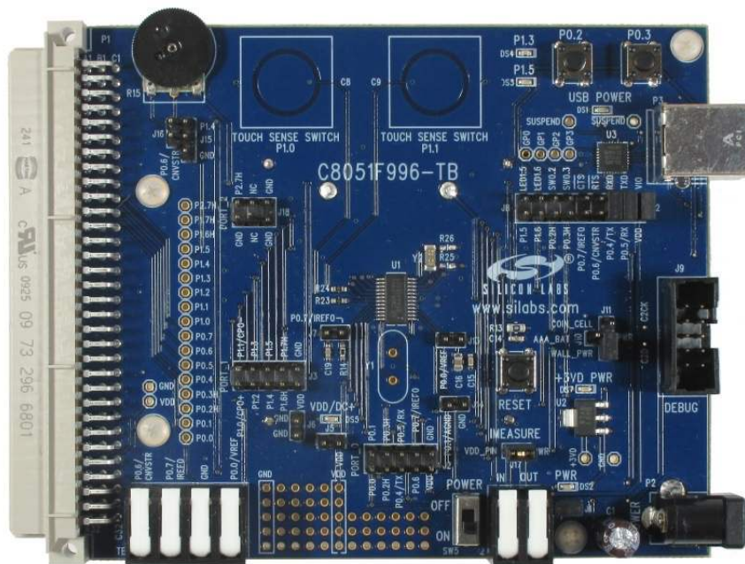
Figure .1. Example C8051Fxxx Development Board
