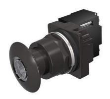
30mm BlackMax, Epoxy Coated Corrosion Resistant Complete Metal Unit Illuminated Push-Pull Operator Transformer type, 480V AC Incandescent Lamp Mushroom Head Cap Small 1 3/4" (44.5 mm) Metal, Black with Clear Lens 3 Position Momentary UL Listed, CSA Certified NEMA 1,3,3R,4,4X,12,13 & Automotive Standards
