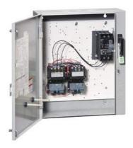
2-speed 3-phase motor starter, Size 0, Two separate windings, Constant or variable torque, Solid-state overload relays, Low spd OLR range 0.25-1A, High Spd OLR range 0.75-3.4A, 110V 50Hz / 120V 60Hz coil, Combination type, 3A circuit breaker, Enclosure NEMA type 1, Indoor general purpose use
