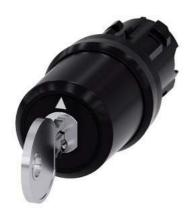
key-operated switch Siemens, 22 mm, round, plastic, lock number SSG10, with 2 keys, 3 switch positions I-O-II, latching, actuating angle 2x45°, 10:30h/12h/13:30h, key removal O+I, with laser labeling, lower case
