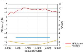
$\bullet$  Tested antenna has been soldered. Evaluation board size is 50x15x1 mm.
