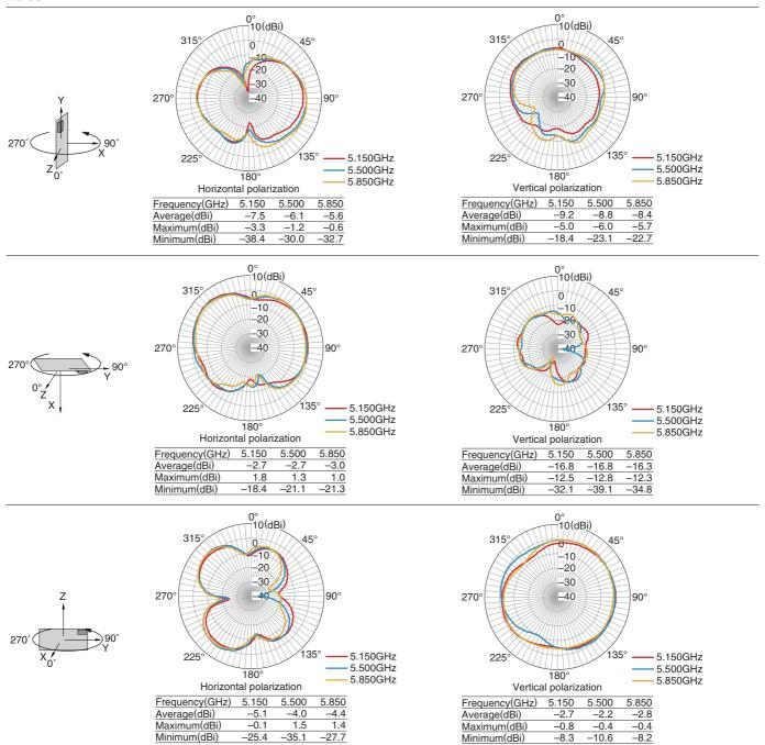
• Tested antenna has been soldered. Evaluation board size is 50x15x1 mm.
