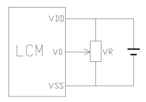
VDD~V0: LCD Driving voltage
