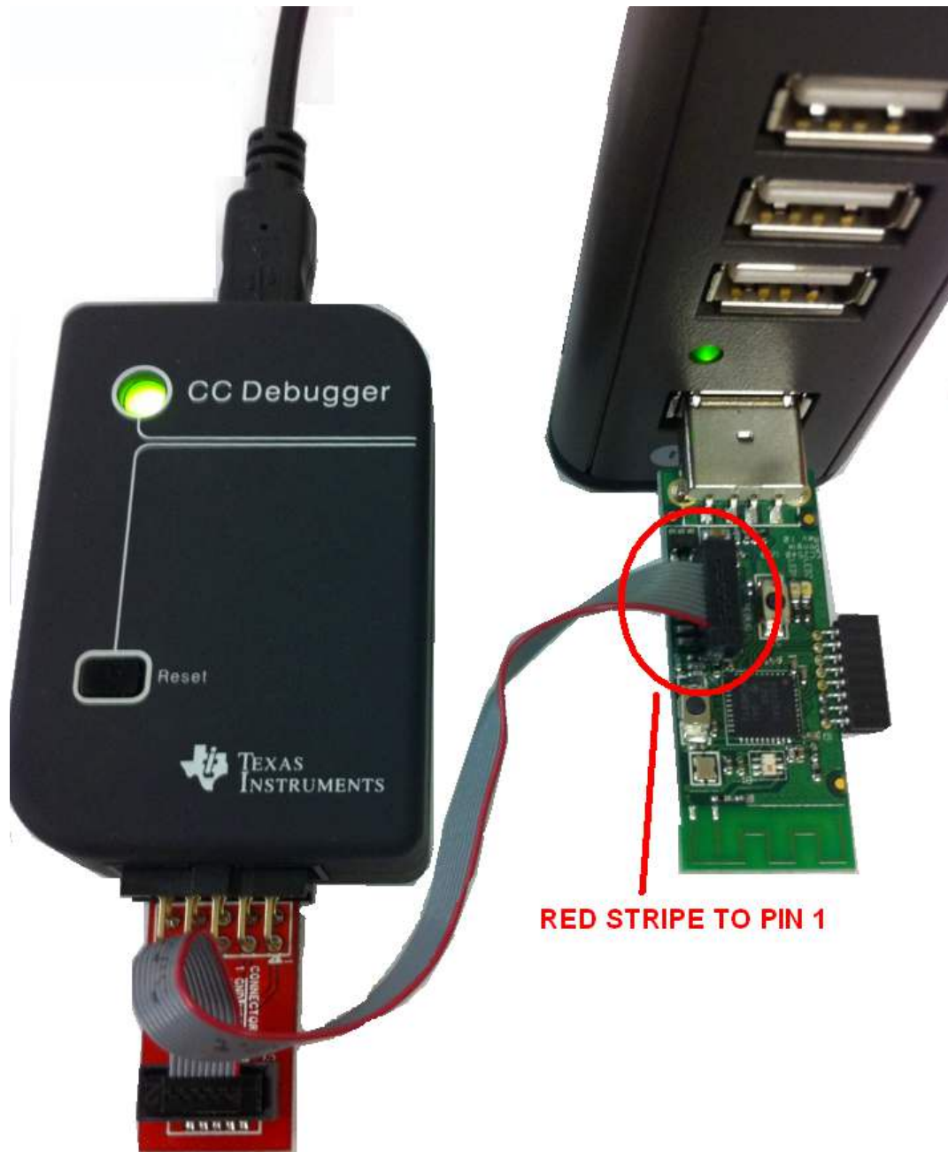
Figure 6-2. CC2540 USB Dongle Connected to CC Debugger
