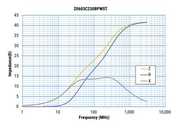
Power Line Ferrite Chip Beads Z-PWS
