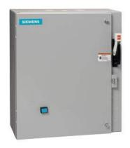
2-speed 3-phase motor starter, Size 0, Two separate windings, Constant or variable torque, Solid-state overload relays, Low Spd OLR range 0.75-3.4A, High Spd OLR range 3-12A, 110V 50Hz / 120V 60Hz coil, Combination type, 30A disconnect switch, Enclosure NEMA type 1, Indoor general purpose use
