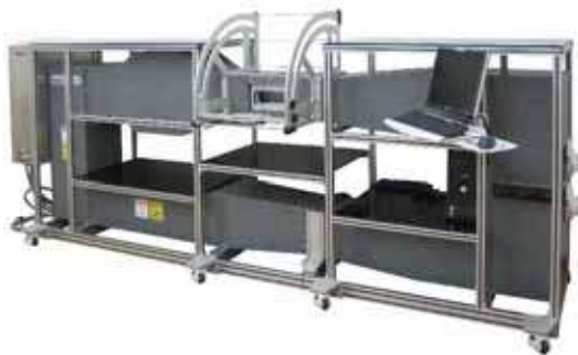
Fig. F: FDK Original Wind Tunnel
