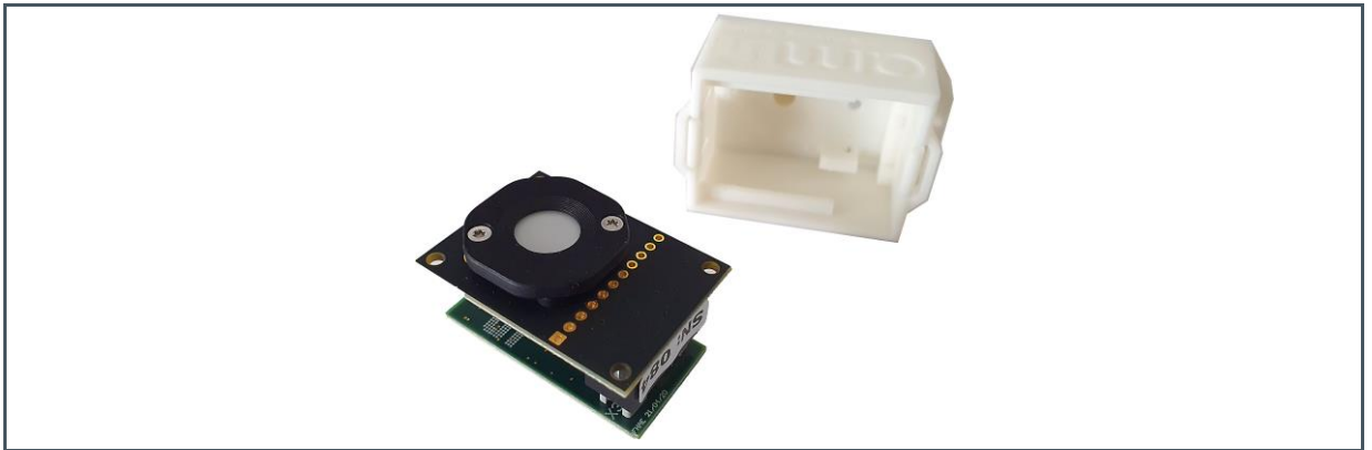
Figure 7: Sensor and Tiny Board Directly Plugged with a USB-Interface, and Plastic Housing
