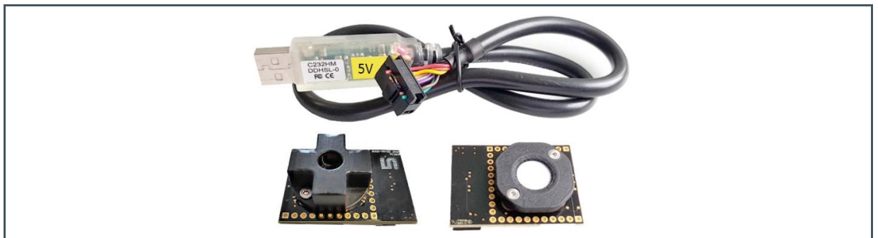
Figure 8: Evaluation Kit with the Sensor Hardware, Optical Adapters (Front), and FTDI Adapter (1)
