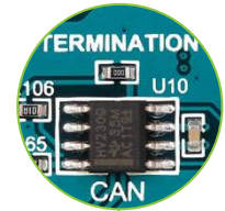
Figure 16-2: CAN transceiver with Node TERMINATION jumper
