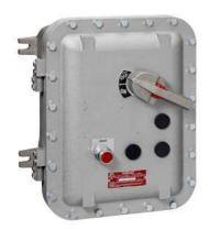
Non-reversing motor starter Size 0 Three phase full voltage Solid-state overload relay OLRelay amp range 3-12A 110V 50HZ / 120V 60HZ coil Combination type 10Amp circuit breaker Encl. NEMA type 4X Fiberglass Water/dust tight noncorrosive Standard width enclosure
