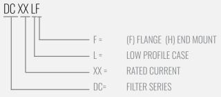
NOTE: USE ANY COMBINATION OF -X (AMPS) WITH ANY -Y RATINGS E.G. **DC100 LF**(100 AMPS, LOW PROFILE CASE, FLANGE MOUNT)
