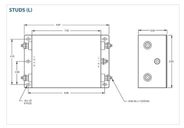
TYPICAL TOLERANCE: +/-0.02" (0.50MM)
