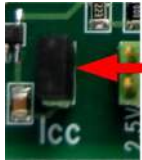
Figure 2.6: Measure power consumption
