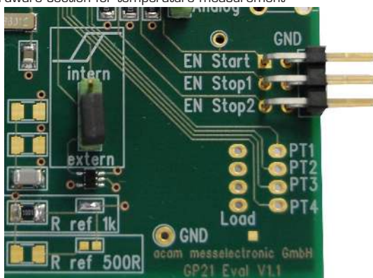
Figure 2.14: Hardware section for temperature measurement
