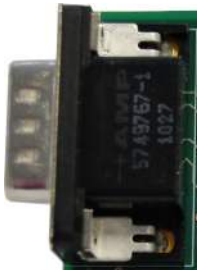
Figure 2.7: 15-pin VGA connector for power supply and data communication via PICOPROG 2.0
