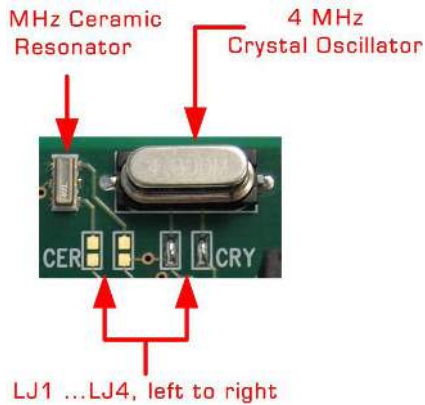
Figure 2.2 High speed clock sources and solder connectors
