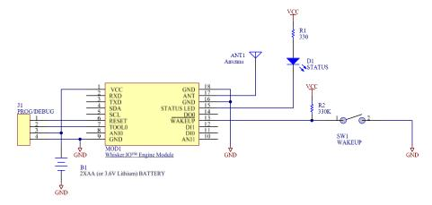
The Whisker.IO Engine is essentially a wireless IoT sensor in a module. Because it can measure temperature internally, all that is required to turn the module into a complete wireless temperature sensor is battery power and an antenna.
