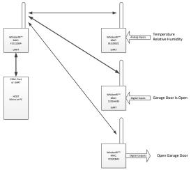
In this example, a master (on the left) is connected to a host (microcontroller or Windows/Linux PC). Three additional modules operate as stand-alone wireless I/O devices. The top right module is connected to analog sensors, the middle right module is using its digital outputs to monitor the state of a garage door, and the lower right module is using its digital output to actually control the garage door.
