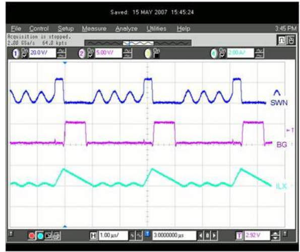
Figure 23. Switcher Operation – DCM Mode
