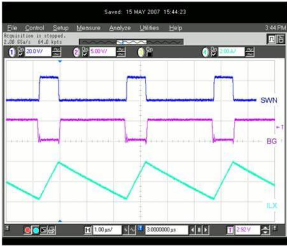
Figure 22. Switcher Operation – CCM Mode
