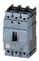
circuit breaker 3VA5 UL frame 125 breaking capacity class M 35kA @ 480 V 3-pole, line protection TM230, FTAM, In=25A overload protection Ir=25A fixed short-circuit protection Ii=6...12 x In cable connection on both sides
