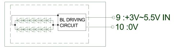
PIN10 is connected to PIN2(VSS) internally
