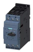
Circuit breaker size S2 for starter combination Rated current 32 A N-release 416 A screw terminal increased switching capacity
