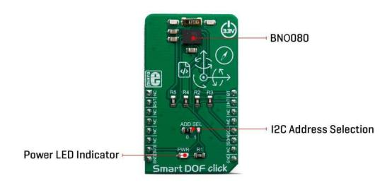
As a device built to be used primarily in smartphones, BNO080 brings events detection and classification system. Stability classification distinguishes among three stability classes: "on the table" (the device is at a fixed position), "stable" (held in hand but in a stationary manner), or at "motion" (the device is in motion). Stability classification is not the only classification for this device. For more information, please refer to the datasheet of the BN080 SiP.
