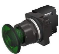
30mm BlackMax, Epoxy Coated Corrosion Resistant Complete Metal Unit Illuminated Push-Pull Operator Full Voltage, 120V AC/DC Incandescent Lamp Mushroom Head Cap Small 1 3/4" (44.5 mm) Plastic, Green 2 Position Maintained, Pull-to-Release UL Listed, CSA Certified NEMA 1,3,3R,4,4X,12,13 & Automotive Standards
