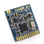
433MHz wireless ISM transceiver module
