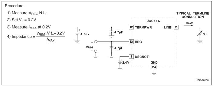
Figure 1. Termline Impedance Measurement Circuit
