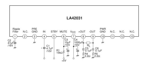
\* LA42031 employs the zero-bias type input circuit, with the input pin potential being nearly zero (about 0.01V). Accordingly, the polarity must be determined according to the DC potential of a circuit connected to the previous stage of LA42031.
