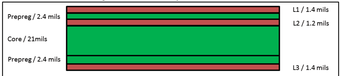
Figure 18: PCB stack-up recommendation
