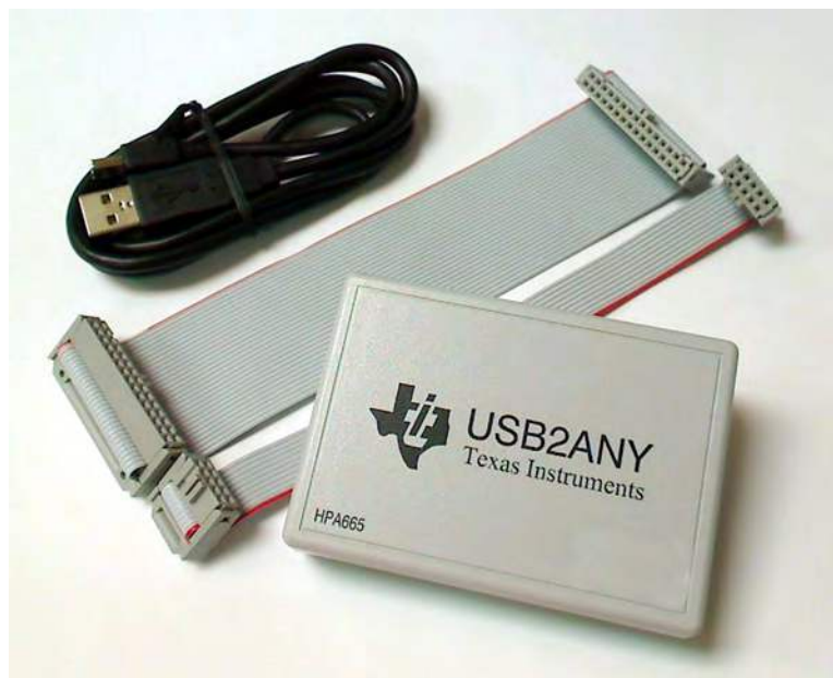
Figure 1. USB2ANY and the Supplied Cables
