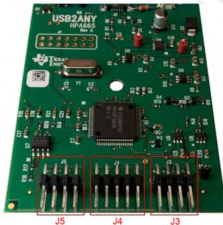
Figure 12. USB2ANY Interface Connectors
